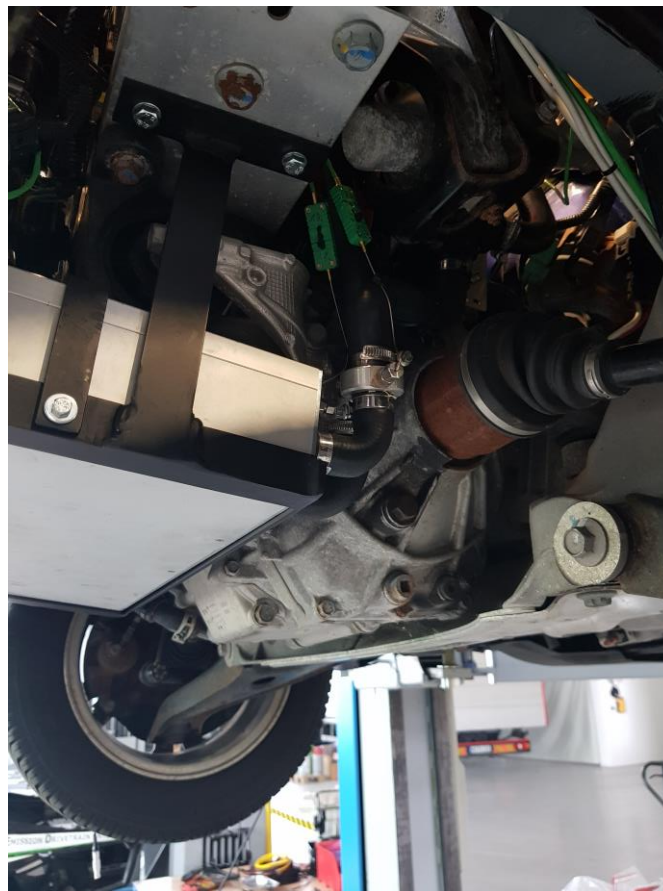
Figure 16: Heat storage tank, prototype integrated in the vehicle
