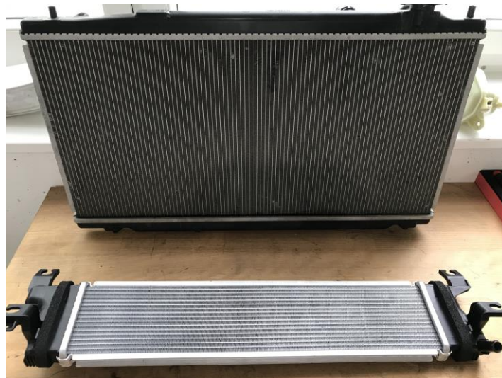
Figure 12: The main cooling radiator and one of the additional radiators
