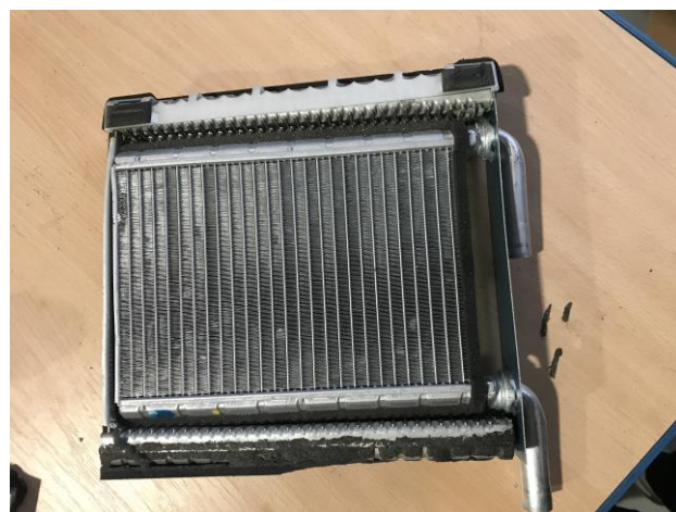
Figure 18: Using the old evaporator as a frame
