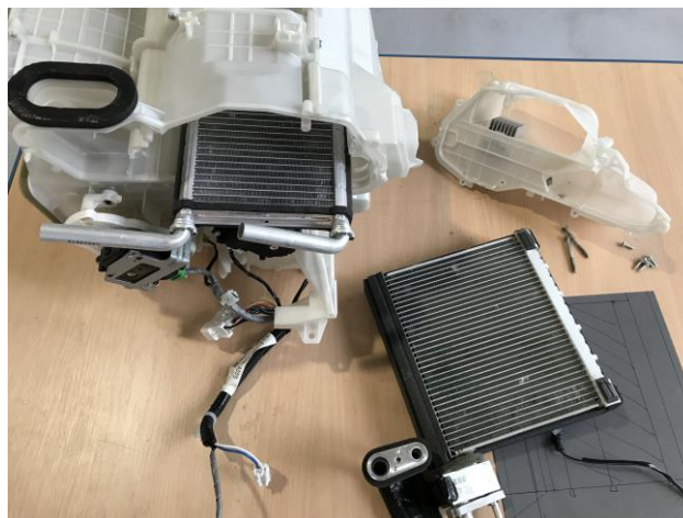
Figure 17: Replacing the evaporator in the HVAC unit
