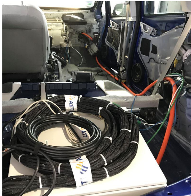
Figure 20: HV power supply and ATT's control box for the IR heating films
