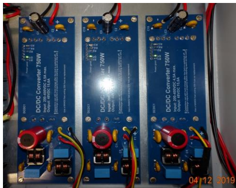
Figure 9: left: DC/DC converter modules; right: three sections with power boards
