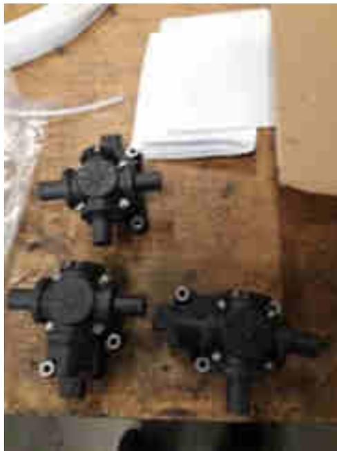
Figure 86: Switching valves to be used in QUIET thermal management system set-up
