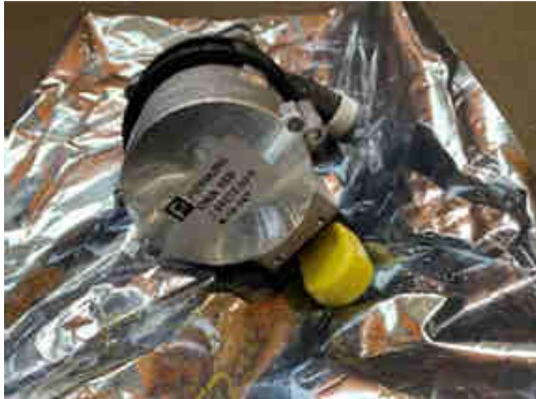
Figure 87: Coolant pump to be used in QUIET thermal management system set-up
