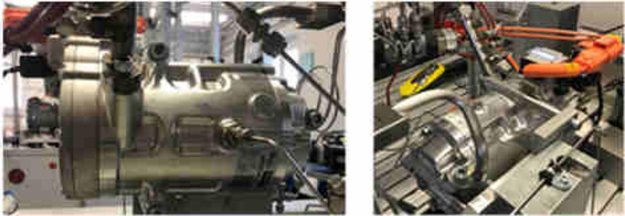
Figure 37: Compressor mounted at test rig for initial testing
