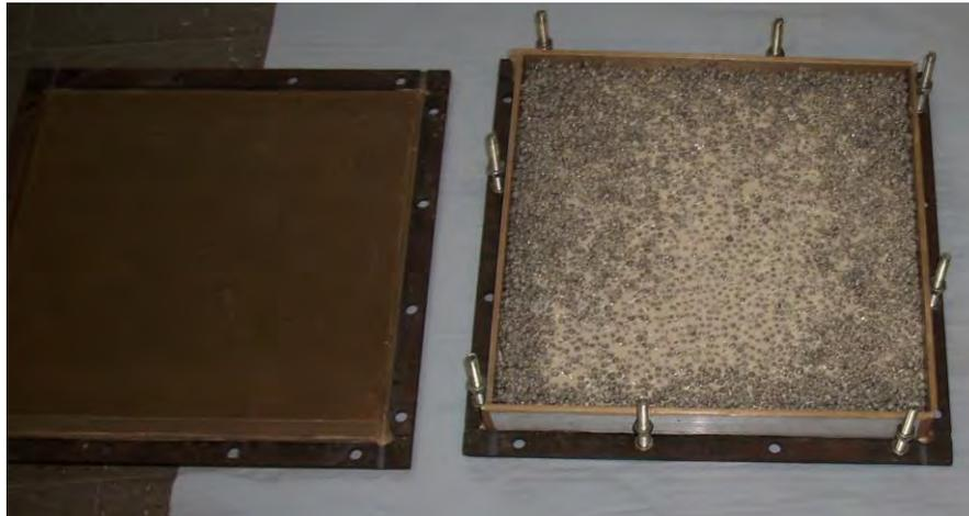
**Figure 4:** Mixture of APM aluminium foam spheres and epoxy system, filled into the mould
