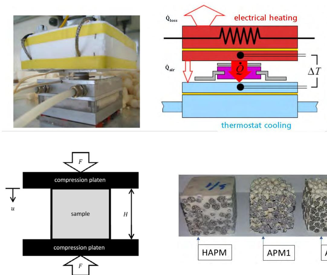
**Figure 3:** Divided bar apparatus for measurement of the thermal conductivity (top left) and schematic sketch (top right). Adjustment of compressive mechanical properties (bottom left) and investigated cubes (bottom right)
