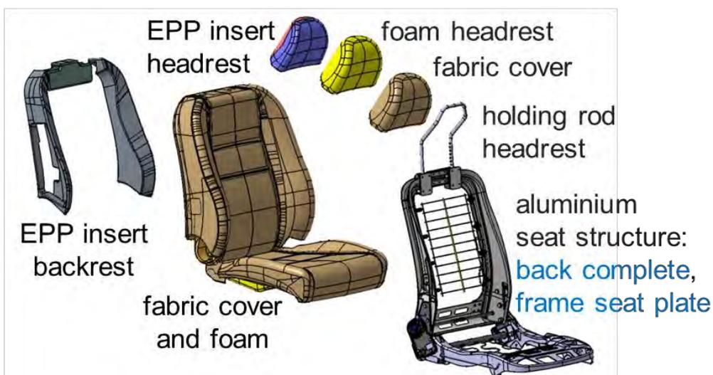
**Figure 12:** New aluminium / steel seat structure with Expanded Polypropylene (EPP) insert in foam
