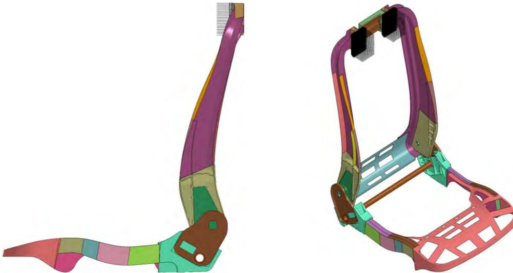
**Figure 18:** Uniformly distributed nodal forces in FE-model of the car seat. Unlike Figure 13 (right), the mesh cannot be seen because the mesh is turned off for a better visualization of the loading.
