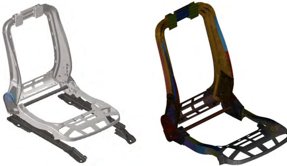
**Figure 13:** CAD model of the seat geometry (left) and FE-model of the seat geometry (right)
