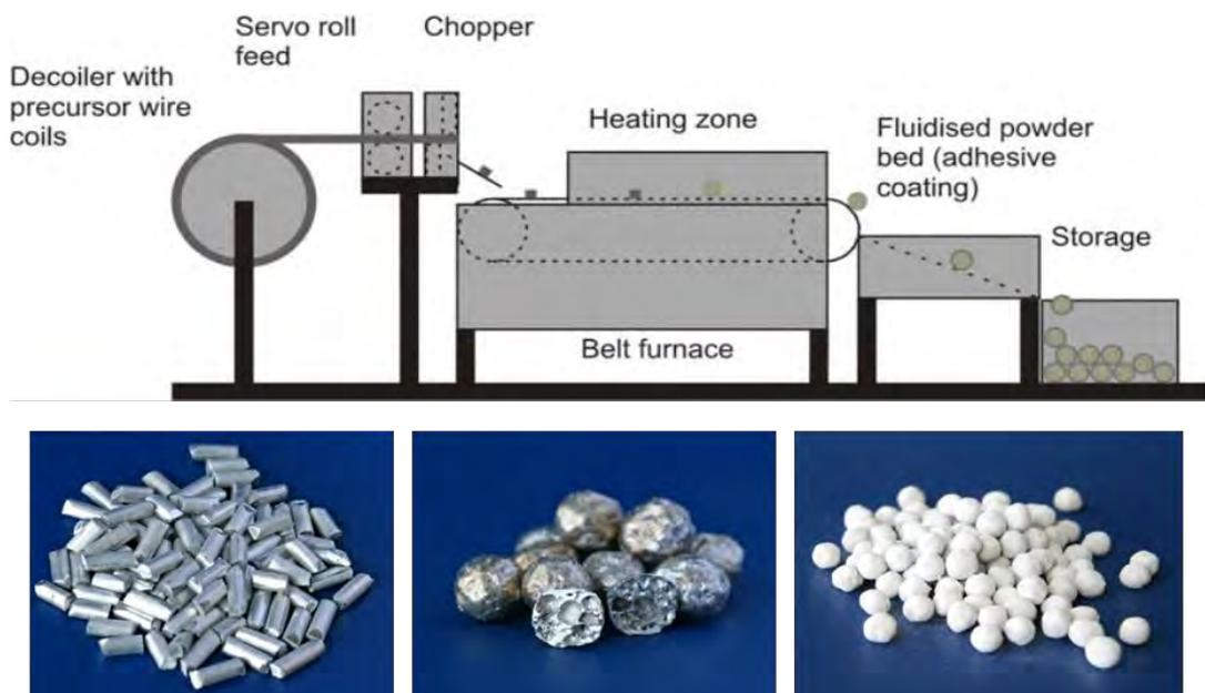
**Figure 1:** Preparation of uncoated and coated APM aluminium foam spheres
