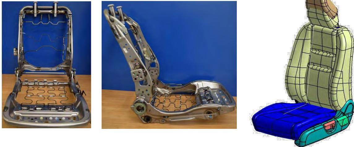
**Figure 8:** Current seat structure in steel (left) and positioning of components as a group in CAD (right).
