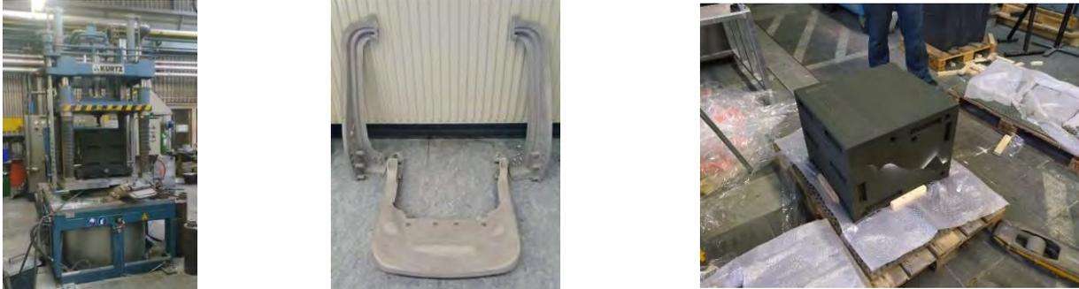
**Figure 20:** LPDC-process (left), pre-burred seat frame components (center) and the two assembled mould halves (right)
