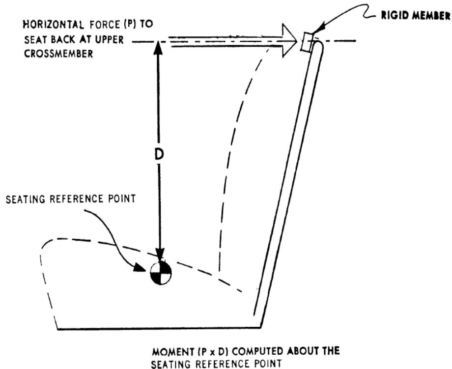
**Figure 17:** Loading scenario according to FMVSS 501.207 [3]
