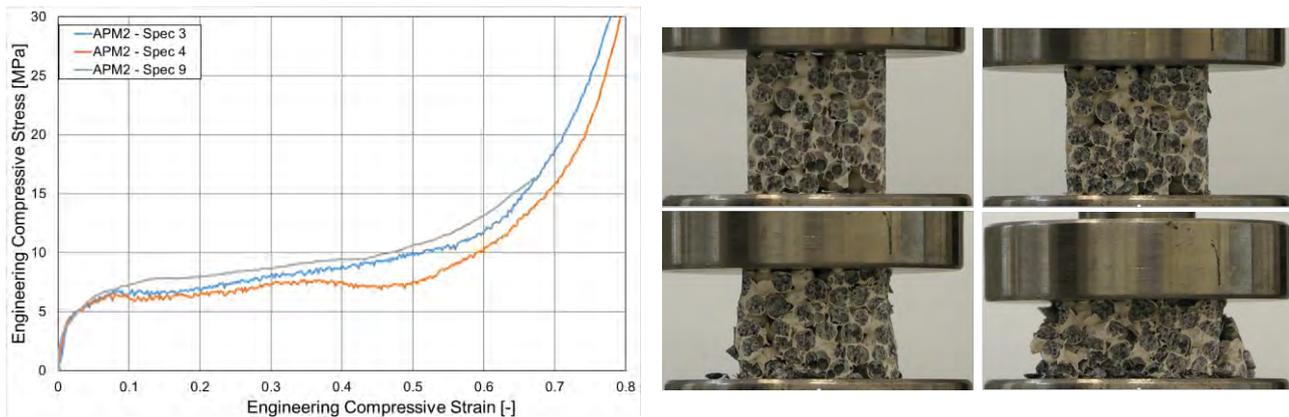
**Figure 7:** Typical stress-strain curves (left) and typical failure (right) of APM2 samples (ECON)
