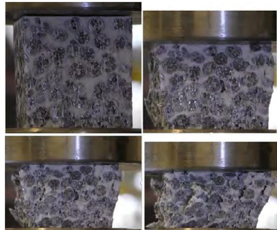
**Figure 5:** Typical stress-strain curves (left) and typical failure (right) of HAPM samples (ECON)
