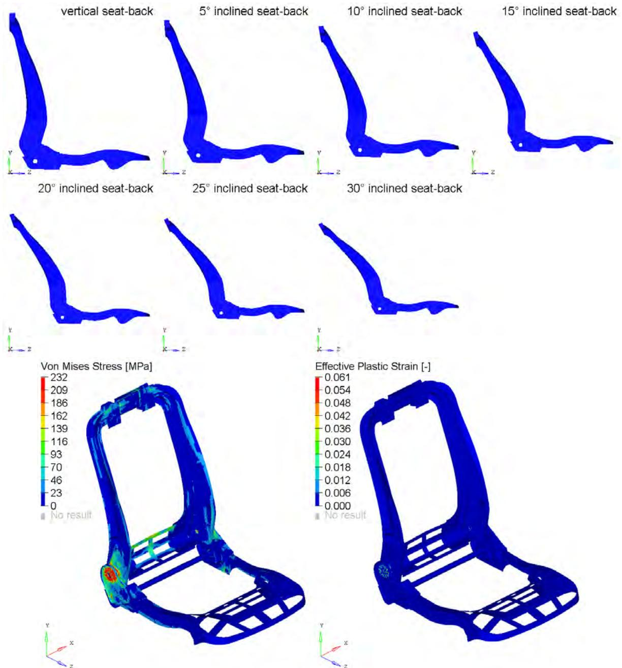
**Figure 19:** Different position of the seat-back (top and middle) and identified worst-case at 5° inclination (bottom left and right)
