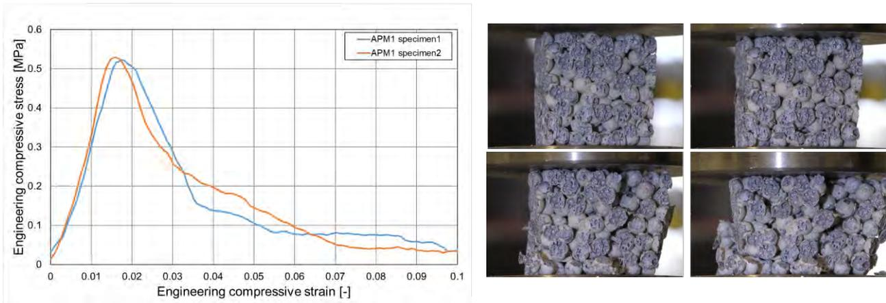
**Figure 6:** Typical stress-strain curves (left) and typical failure (right) of APM1 samples (ECON)
