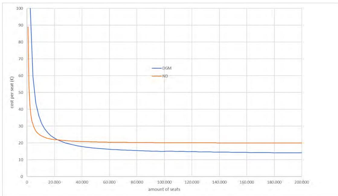
**Figure 23:** Cost of cast parts per seat vs. amount of seat structures, comparing LPDC (orange line) and HPDC (blue line) technique.
