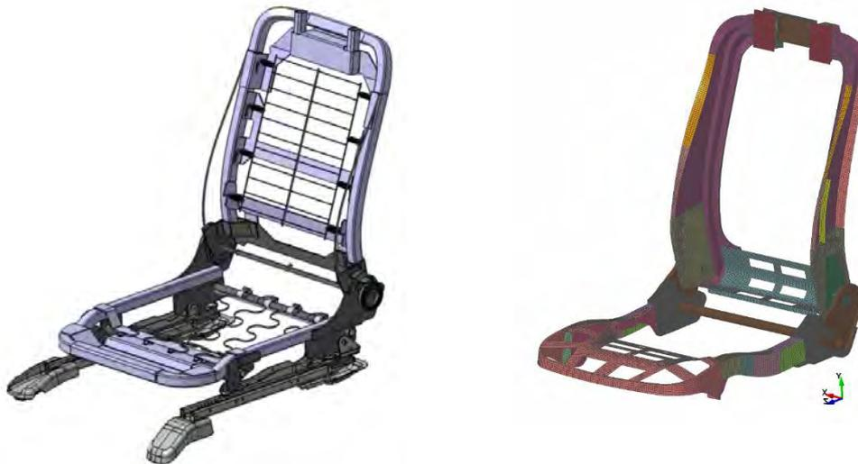
**Figure 10:** Stages during design phase. Left: 1<sup>st</sup> iteration (aluminium parts in blue, steel parts in grey colour), Right: final aluminium steel seat structure.
