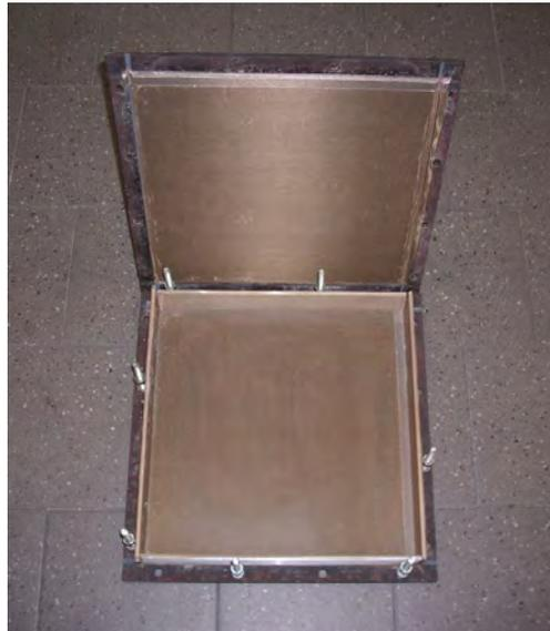
**Figure 2:** Steel mould for preparing samples of dimensions ca. 300 x 300 x 35 mm
