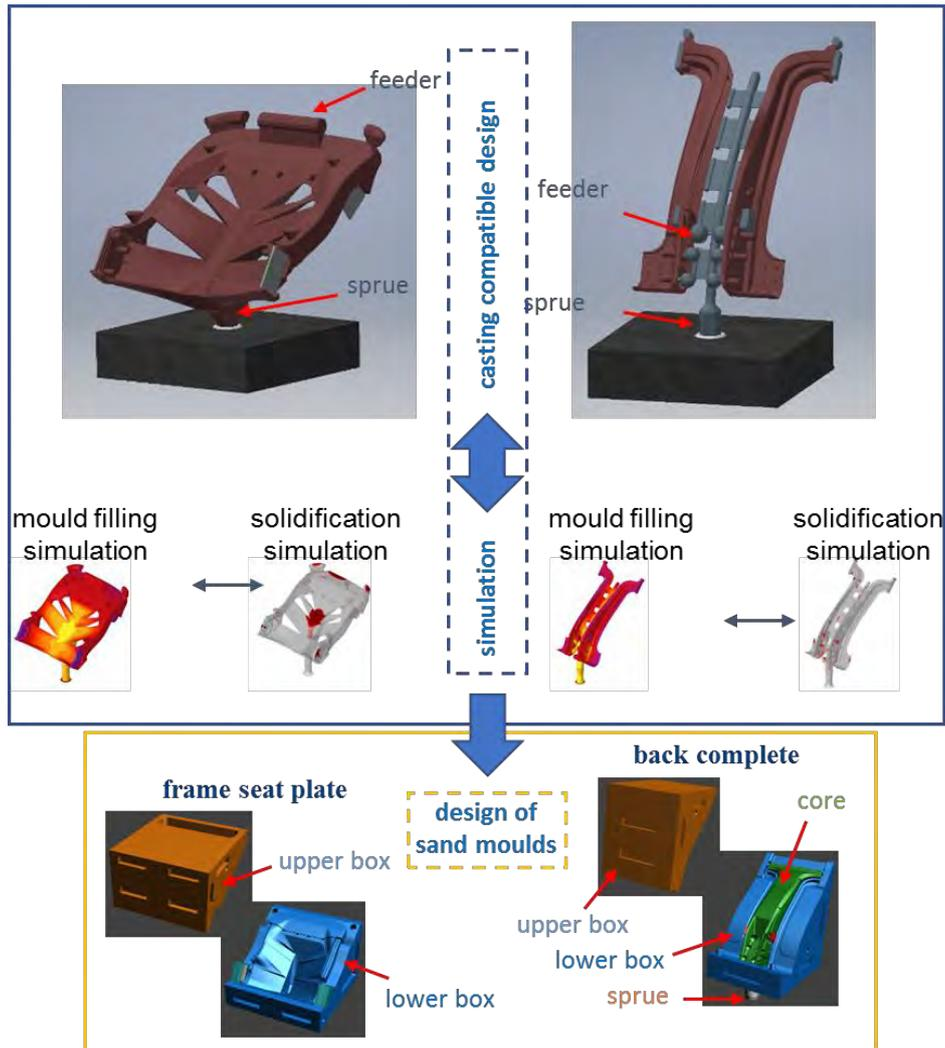
**Figure 21:** Summary of preparatory works: casting compatible design for the cast parts, mould-filling and solidification simulation and design of casting sand moulds.
