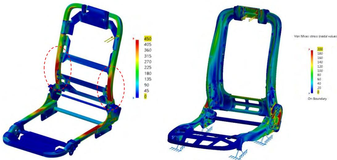
**Figure 11:** Test of strength results during CAD-design phase for 1<sup>st</sup> design iteration (left) and final lightweight aluminium steel seat structure (right).
