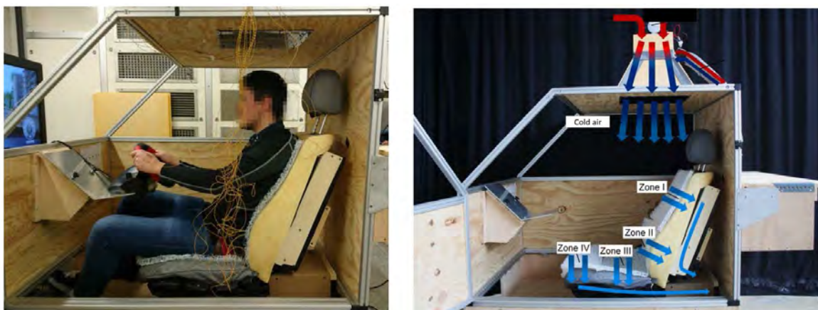
Figure 19: Experimental setup of "cold air shower" [55]
