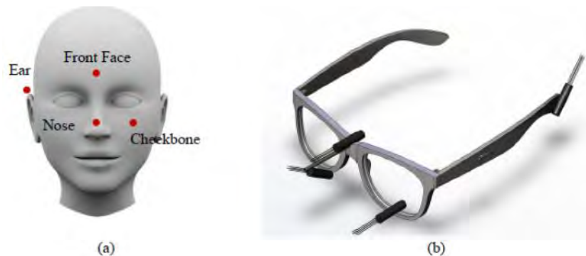
Figure 12: (a) infrared sensing locations, (b) sensing device with sensors [48]
