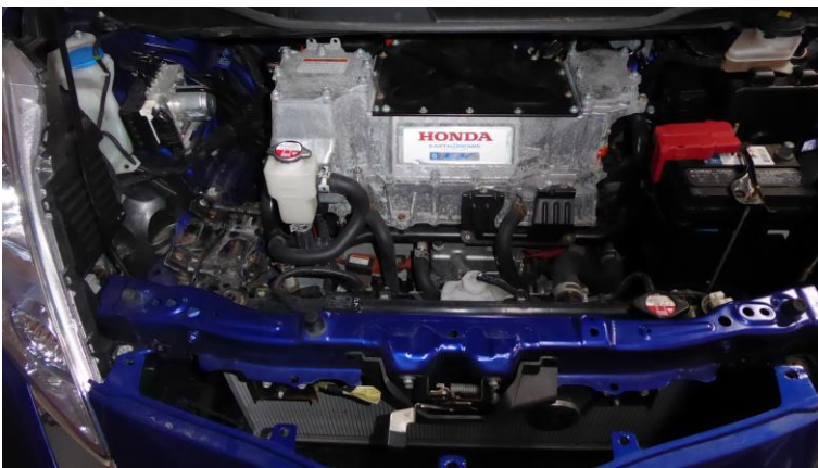
Figure 4: Engine bay of the Honda Fit EV without A/C components
